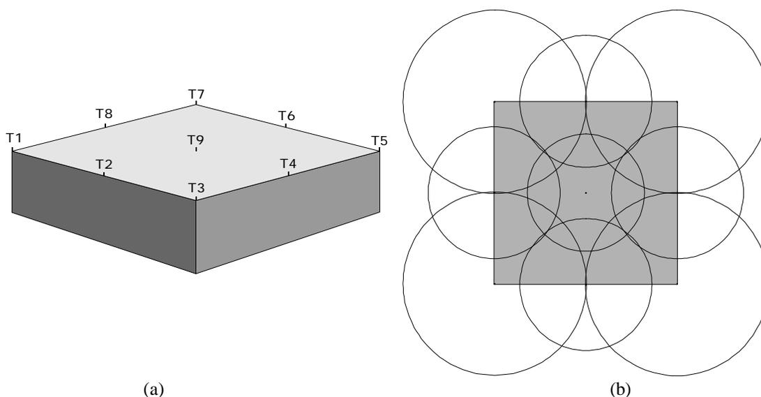
**Figure 3:** Example of the Collection Volume design method. Protection of a building 20 m high and 50 m wide and deep, using conventional finials 1 m high, 15 mm in diameter and with a tip radius of curvature of 1 mm. (a) 3D view. (b) Plan view.
